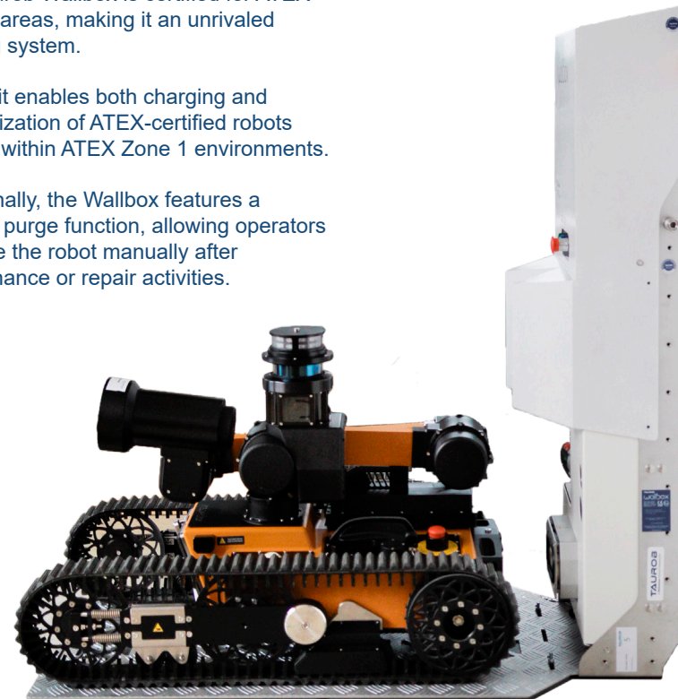
The floor plate is designed to be stepped on and optimized to handle various ground conditions, ensuring stability and durability in harsh industrial settings
