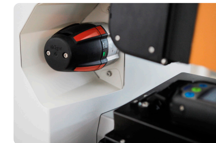
Integrated gas sensor Polytron for safe charging of the Dräger X-am 8000 gas detector on the robot
